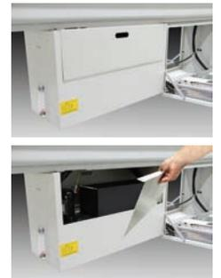
Access to remnant pan from both sides of bar feeder for easy remnant removal.
